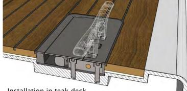
Installation in teak deck on welded metal structure or GRP (reinforced by metal inlay). Screwing in threaded blind hole.
