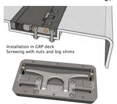
Complete unit as delivered top plate and pivoted cover shown as white lines (subject to change without notice)
