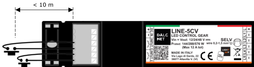
Figure 7: Local Command connection diagram for Short Distances
