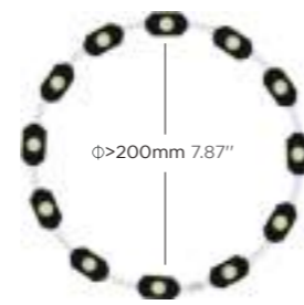
Correct bending way
