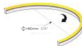
Correct bending way
